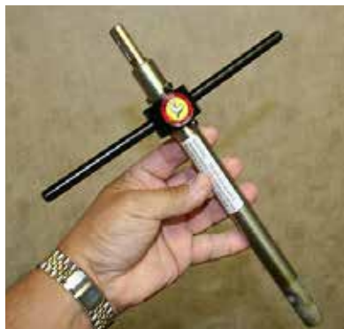
#KL001 Kluge Drill Attachment T-Handle Adapter to be used from StrikeMaster hand auger to electric drill
